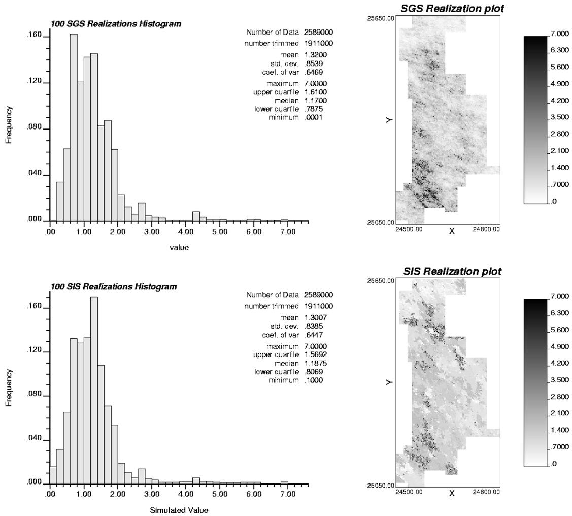
**Figure 3:** SGS (on top) and SIS (on bottom) realizations maps and histograms at a 2m x 2m x 2m grid size.
