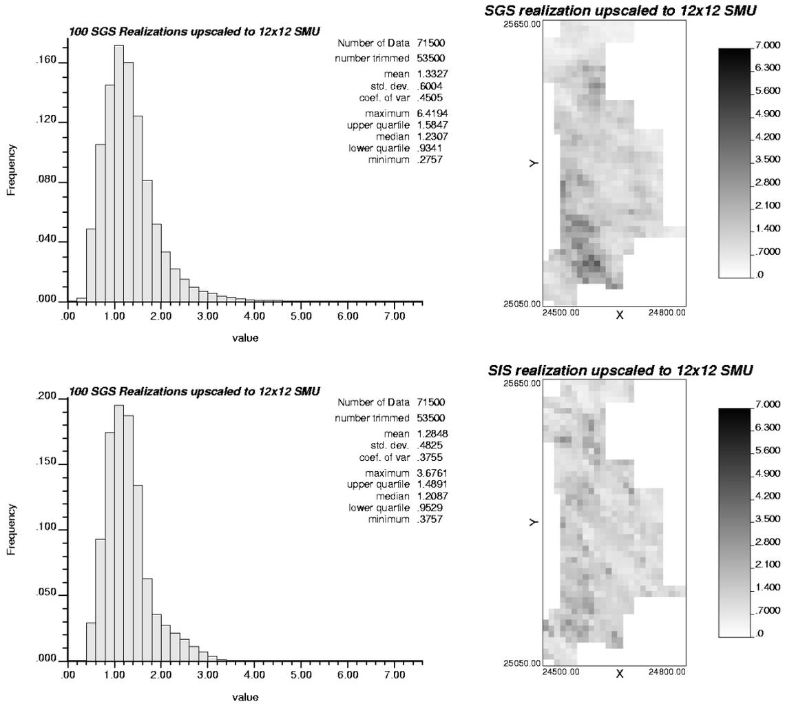
**Figure 4:** Upscaled SGS (on top) and SIS (on bottom) realizations maps and histograms to a 12m x 12m x 12m SMU size.
