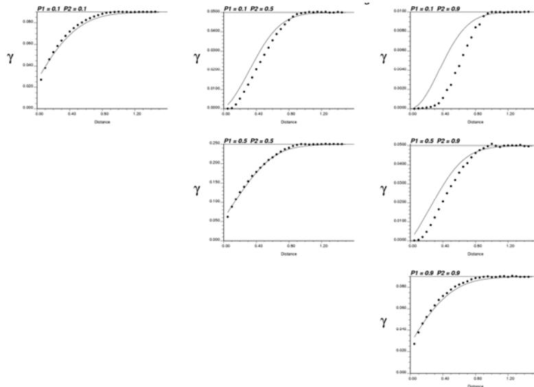
**Figure 6:** Theoretical bigaussian derived indicator direct and cross variograms (dots) and an attempt to fit them with a LMC (continuous lines)
