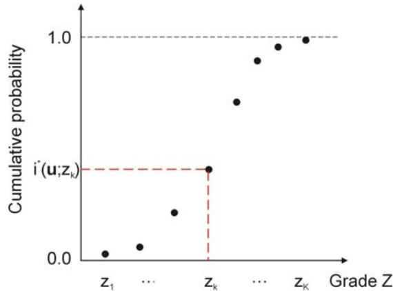
**Figure 1:** Discretized conditional cumulative distribution function at a given location  $\mathbf{u}$ . The estimated indicator value for a cutoff  $z_k$  represents the estimated cumulative probability at that cutoff.
